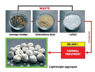
Lightweight aggregate production technology using sewage sludge is safe, Energy efficient, environmentally friendly and cost-effective method for utilization of sewage sludge. Additionally, it provides an attractive building product exclusively from waste materials. The main objective of the Project is to demonstrate innovative waste management of sewage sludge along with silica waste in the process of production of artificial lightweight aggregate
